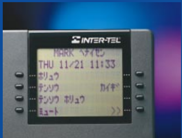
An active outside call is displayed in Japanese along with call duration and approximate call cost.
