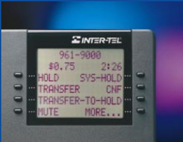
An active outside call is displayed along with call duration and approximate call cost.
