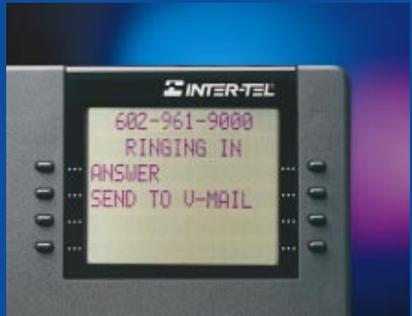
Inter-Tel AXCESS supports Caller I.D. with directory look-up. The system can display a phone number or company name.
